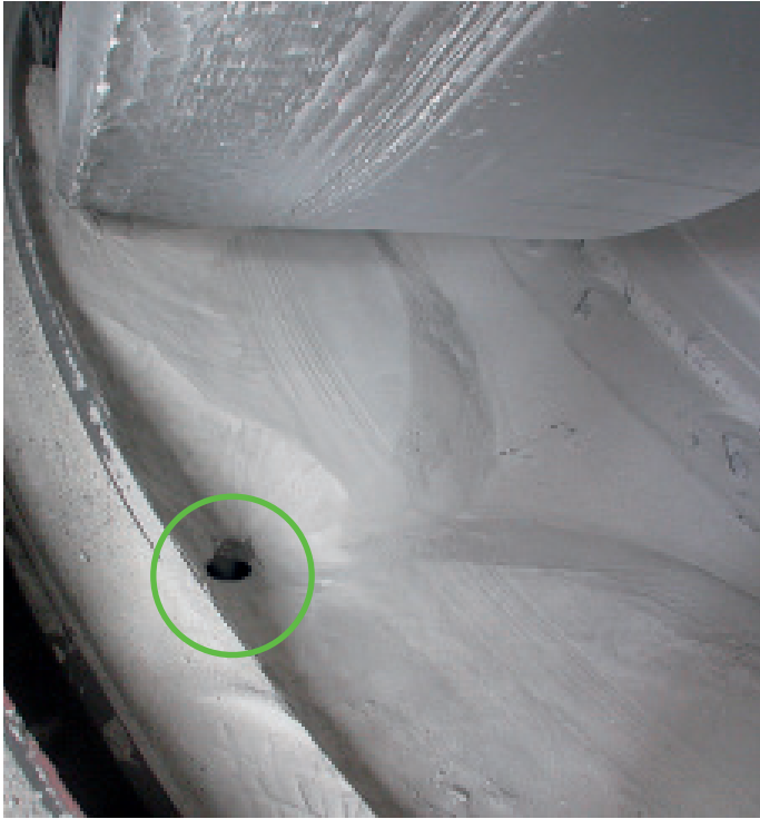
Outlet openings for foreign particles
