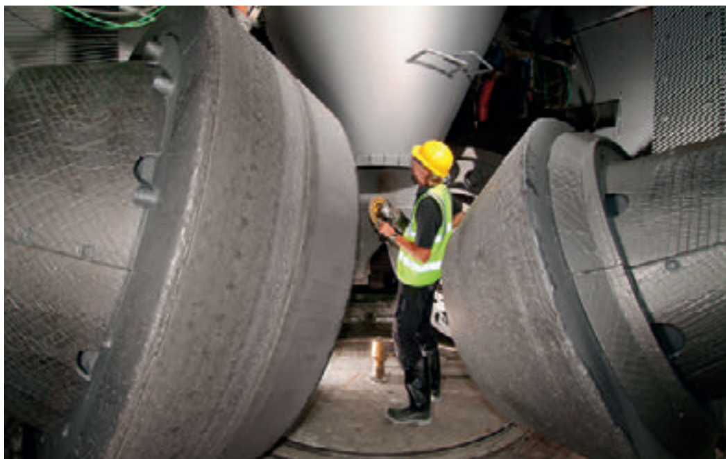
M roller and S roller in working position
