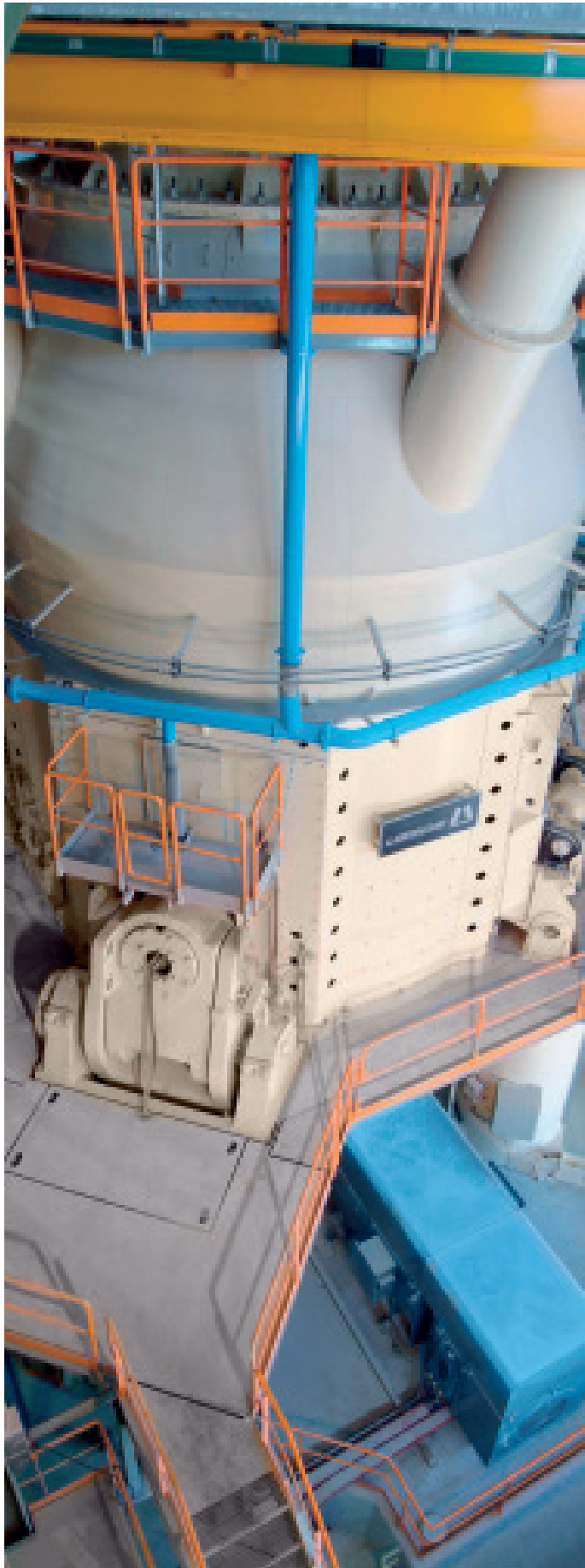
Central grinding plant for granulated blast furnace slag LM 46.2+2, Dunkerque, France, 2005
