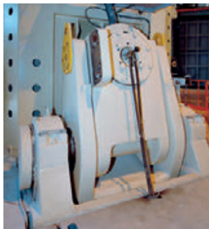
M roller: rocker arm in working position
