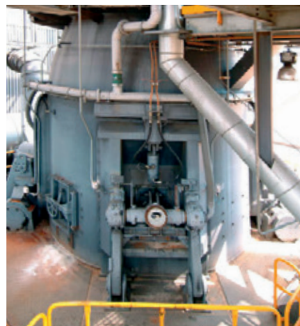
S roller: rocker arm in working position
