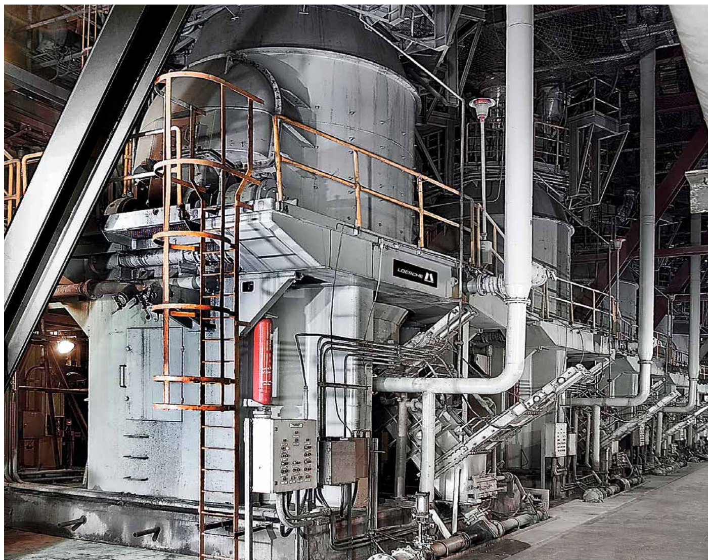
Loesche mills, 10 x Type LM 28.2 D, Taiwan Power Co., Taichung, Taiwan, 2000
