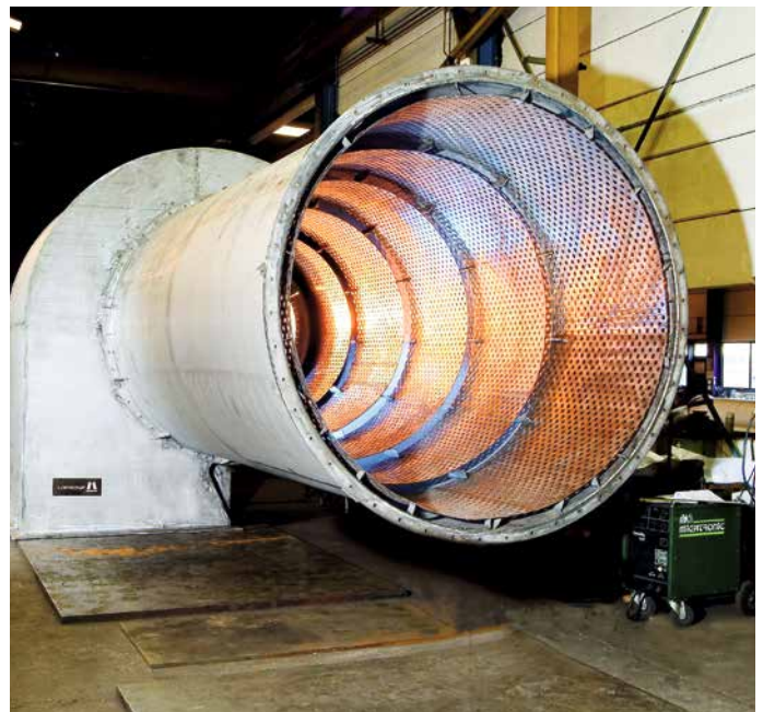
LOMA furnace Type LF 25 for blast furnace gas, for the steel plant Tubarão, Brazil, 2004
