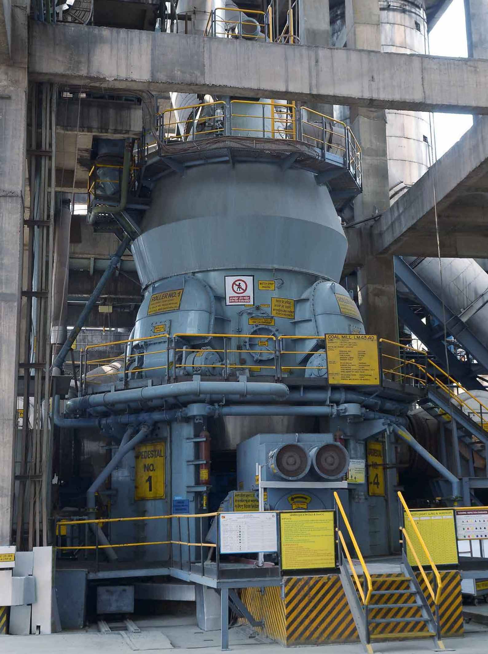
Loesche mill Type LM 43.4 D, in Kotputli, India, 2006
