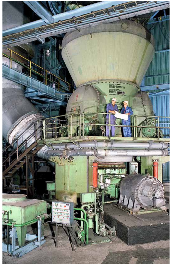
3-roller modular Loesche mill Type LM 28.3 D in Kosice, Slovakia, 1991
