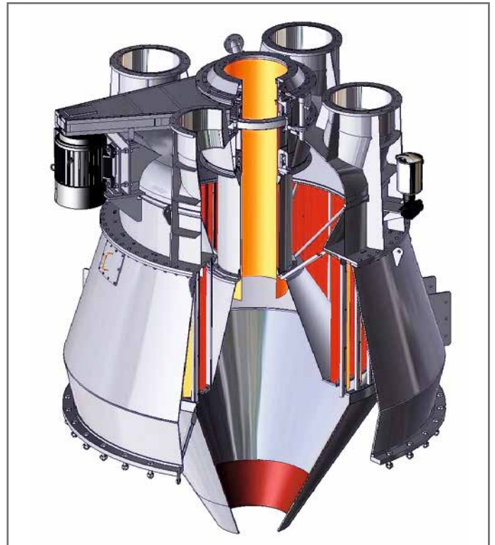
LSKS classifier with central inlet and 4 separate product discharges for direct-firing boiler plants
