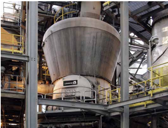
3-roller modular grinding Loesche mill Type LM 28.3 D in Union Bridge, USA, 1999
