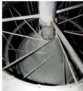
LSKS rotor with replaceable rotor blades
